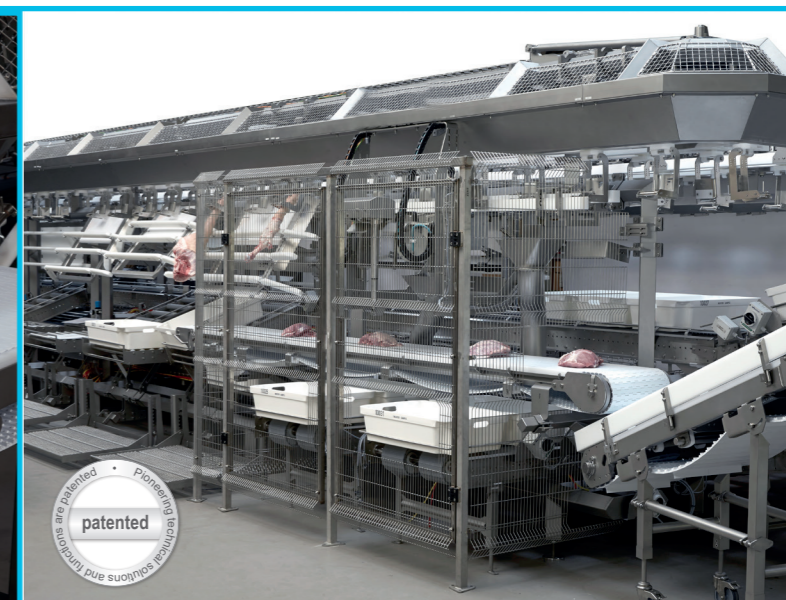
Modular built system with individual working stations and conveyor system
