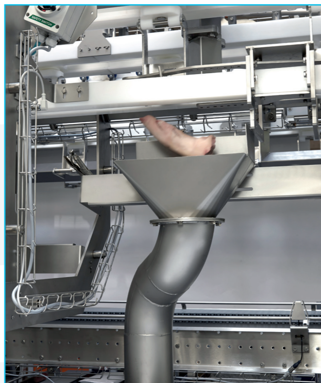
Release of the foot through a funnel into a tray underneath the station
