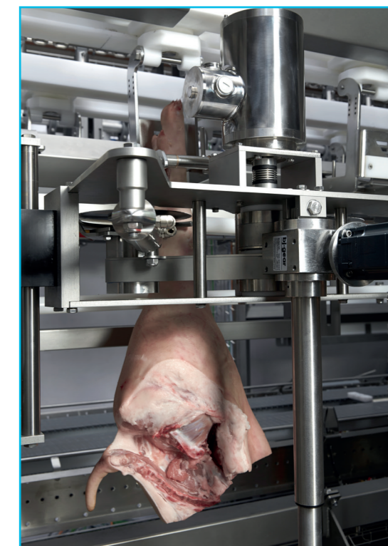
Automatic turning of the product is done during the round cut process
